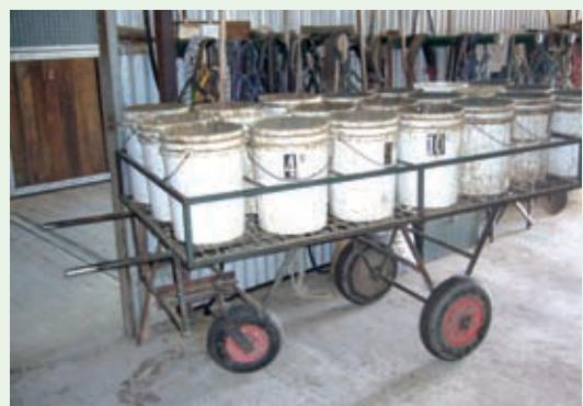
This feed trolley has wheels which allow the trolley to be used over rough terrain in and around the stable.
