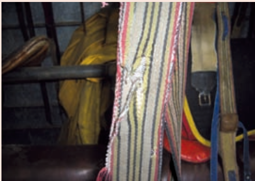
Girth straps – damaged and worn.
