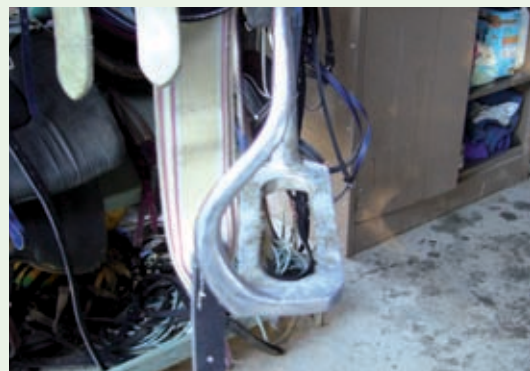
Safety irons used for track work.
