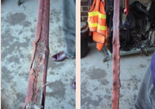
Riding reins – damaged and worn.
