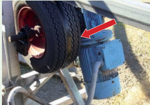
Horse walker drive motors, shafts or belts must be guarded.
