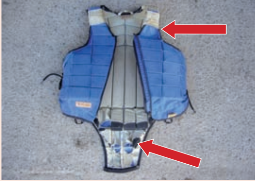
Body protector – damaged with excessive wear.
